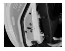
door panel, this may damage your panel. These snaps will make a "pop" sound as they release one by one. Once all snaps have been release the door panel can be lifted. Pull the door panel upwards to remove from the door.
