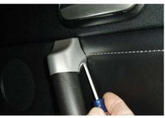
• Gently insert your small flat head screwdriver upwards into the base of the plastic cap at the top of the main door grab handle. Apply upward pressure until the plastic cap comes off into your hands. Be ready to catch these because they have been known to take flight.
