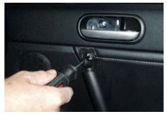
• Locate the screw inside the doors cup holder and remove with your #2 Phillips head screwdriver.
