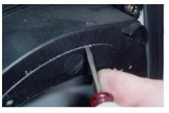
There is a "groove" around the top and bottom of the oval opening that the factory put in place for us to easily be able to install the round CWC-9 speakers. Using the corner of your small flat head screwdriver, score the plastic along
