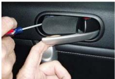
• With the door handle still in the "open-the-door" position, insert the small flat head screwdriver into the front of the now loosened blank plastic insert and pry it out.
