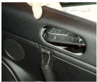
• Remove the connector from the door lock wires on the back side of the door panel. Remove the connector from the factory tweeter. (these connectors can be tricky as they require the insertion of your small sized flat head screwdriver into their "release" tabs as you are pulling them out)
