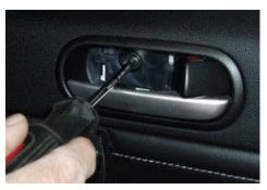
• Using a #2 Phillips head screwdriver, unscrew the screw from behind the blank plastic insert that you just removed.
