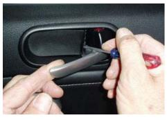
• With the door handle held in the "open-thedoor" position, gently insert a small flat head screwdriver behind the blank plastic insert and apply enough prying force to loosen.
